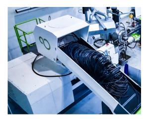
As an all-rounder, the ISEC evo machine processes bulky hose bundles as well as start-up lumps and complete rolls with drip tapes. Photo: PURE LOOP
